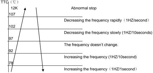
TTC>=107°C lasts for 20 seconds. Overheating protection of air-blowing, alarm malfunction to the indoor, others don't last.
